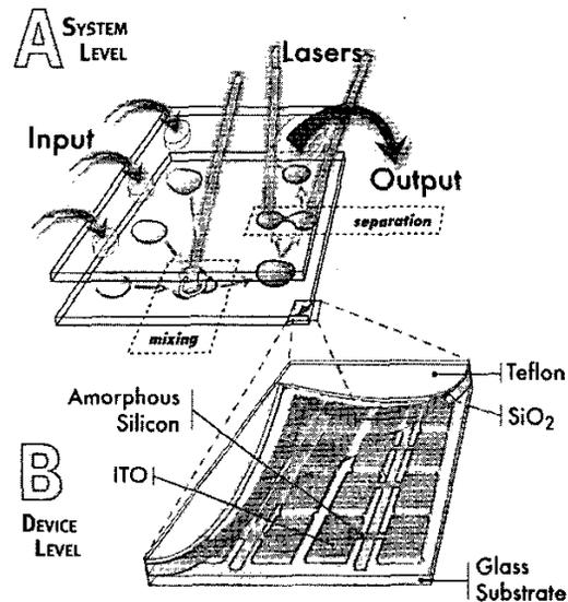
Fig.1(A) Schematic illustration of liquid droplets manipulation in opto-electrowetting (OEW) device. (B) Schematic of the OEW surface
