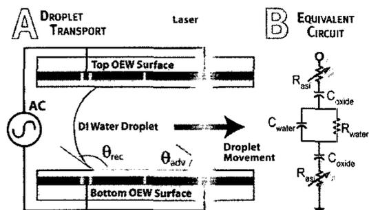
**Fig.2** (A) Illustration of contact angle change on OEW surface. (B) Equivalent circuit for one unit cell of the OEW device.  $R_{asi}$  is the resistance of the amorphous silicon photoconductor under light illumination;  $C_{oxide}$  is the capacitance of the  $SiO_2$  insulator;  $C_{water}$  and  $R_{water}$  are the capacitance and resistance of water layer between the two OEW surfaces.
